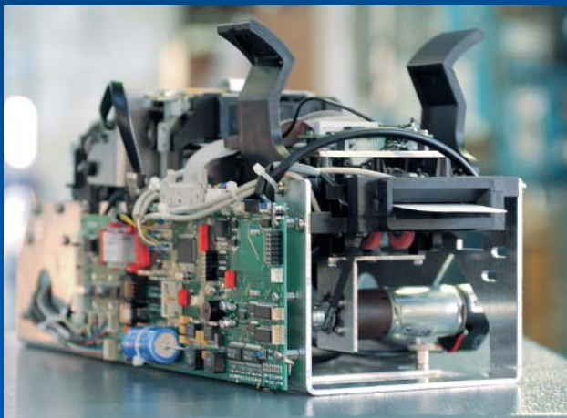
THE TECHNICAL CORE COMPONENT OF THE PM ABACUS DEVICES IS THE MULTICON, THE HIGHLY INTEGRATED TICKET PROCESSING UNIT
